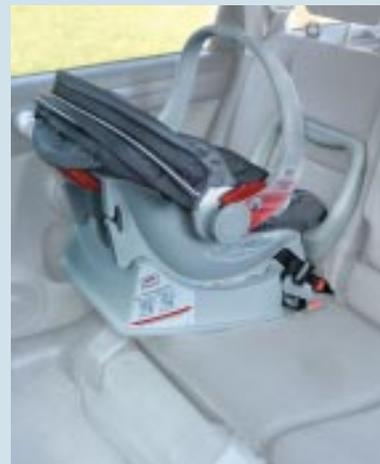
**WORLDS APART** The Britax Cosy Tot, left, sold in Europe, has a "foot" to help stabilize the base, which the Britax Companion sold in the U.S., right, lacks. The Cosy Tot was the top performer in our tests; the Companion performed poorly.
